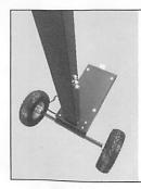
1. Attach wheel assembly to base as shown. Place grey hubcap on shaft, then slide on the 3" sleeve, slide wheel over sleeve, hubcap and finishing nut. Repeat on the other end of shaft.
